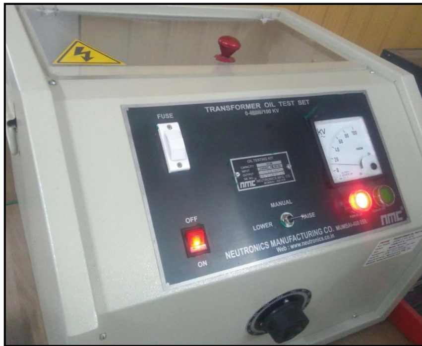
Fig. 4.1 Transformer oil test set
